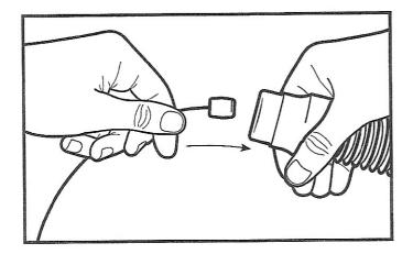
**Step 3:** Continue to feed the weighted end of the Tube Brush into the CPAP tube until the weight comes out the opposite end, and the brush is positioned near the hose outlet.
