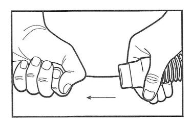
**Step 6:** In one motion, pull the Tube Brush through the CPAP tube as far as possible.
