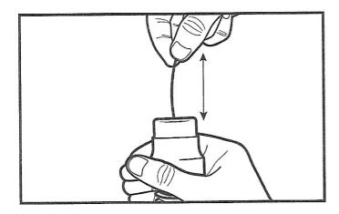
**Step 4:** Use your fingers to push the brush end of the Tube Brush fully into the CPAP hose.
